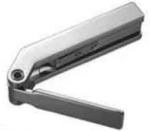
321.120 1 Tension Device, articulated Span 20mm, can also be used as a distractor. Colour scale: yellow up to 500N, green up to 1000N, red above 1000N.
